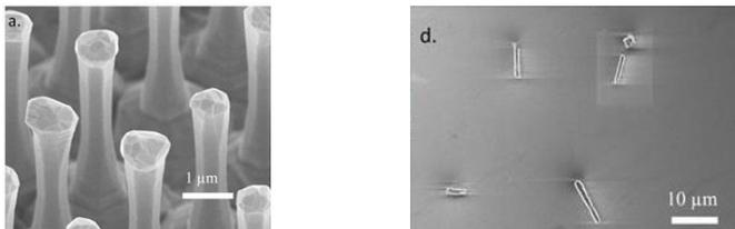
Scanning electron microscopy images of (a) as-grown hex-SiGe and (b) of the nanowires transferred to the substrate.
