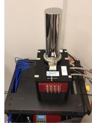
(a) Scanning Electron Microscope image of a superconducting single photon detector (SNSPD). The detector consists of a thin, superconducting wire formed into a meander structure for optimal coupling to the mode of a single mode infrared optical fiber. (b) Image of the 2.3 μm ONCHIPS SNSPD system.
